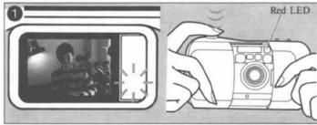
The flash will activate automatically when the shutter release button is fully pressed.
